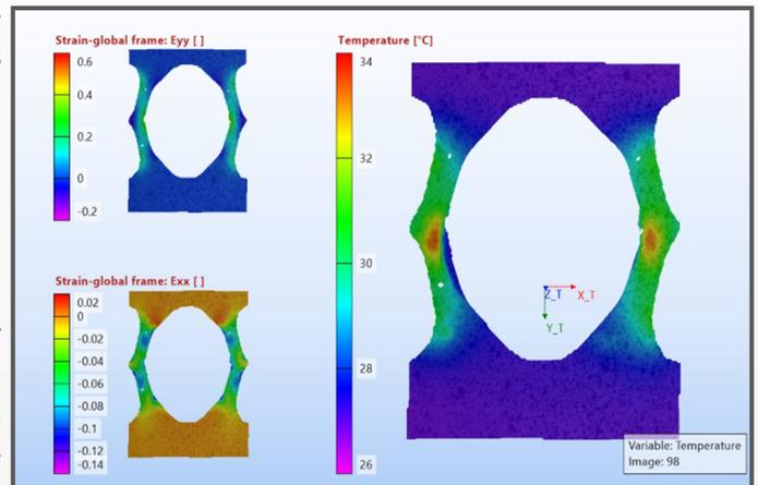
As can be observed, strain concentrations and varying strain rates coincide with a local temperature increase. One can now investigate the relationship between a strain component and the temperature at any point. The compressive transverse strain component reveals an approximate linear behavior with temperature.
